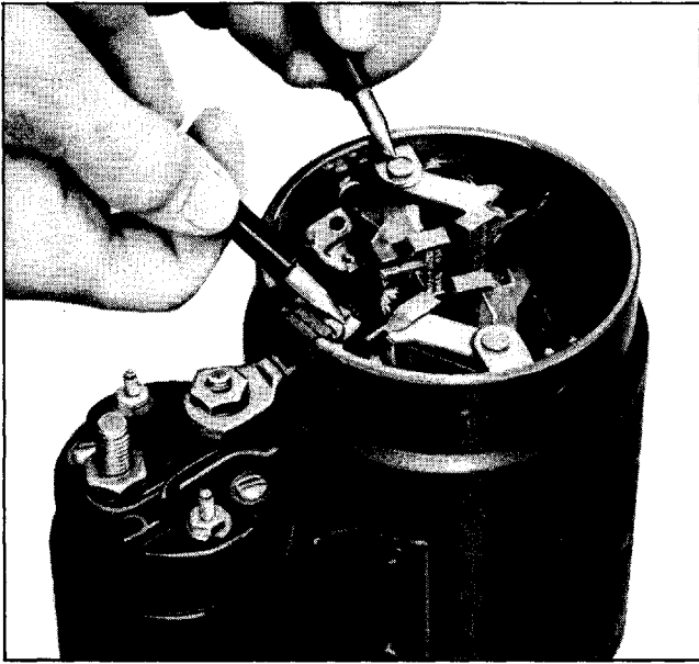
Fig. 12-32 Testing Field Coils for Ground
