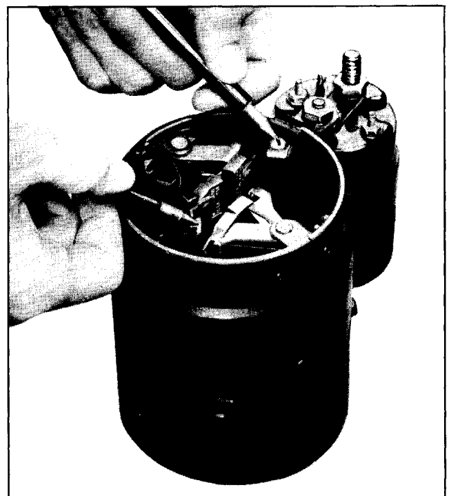
Fig. 12-31 Testing Field Coils for Open Circuit
