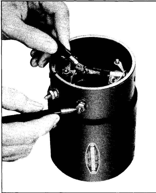
Fig. 12-18 Testing Field Coils for Open Circuit
