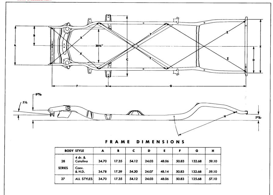
Fig. 2-1 Frame Checking Chart
