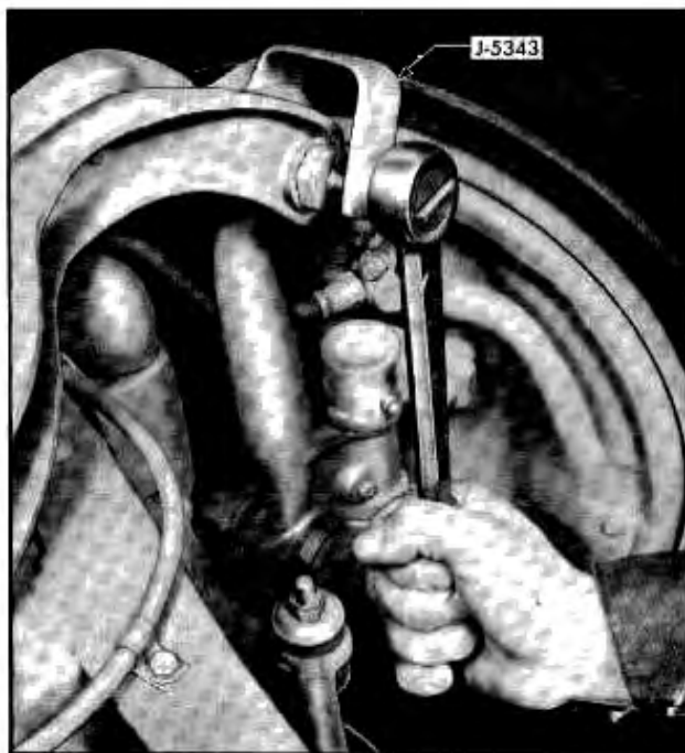
Fig. 3-12 Adjusting Caster or Camber
