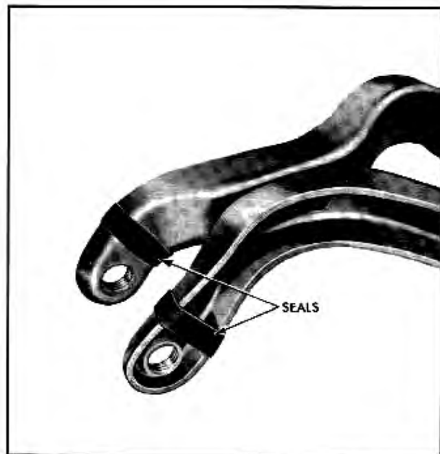
Fig. 3-17 Seals Positioned for Assembly of Pivot Pin
