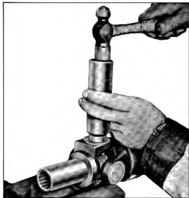
Fig. 4-46 Removing Bearing From Splined Yoke Member
