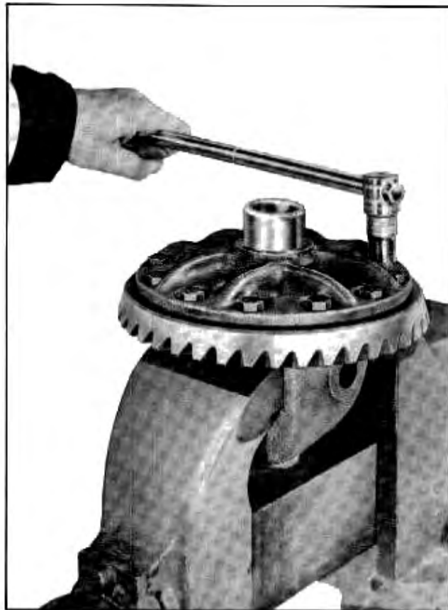
Fig. 4-41 Removing Ring Gear From Case
