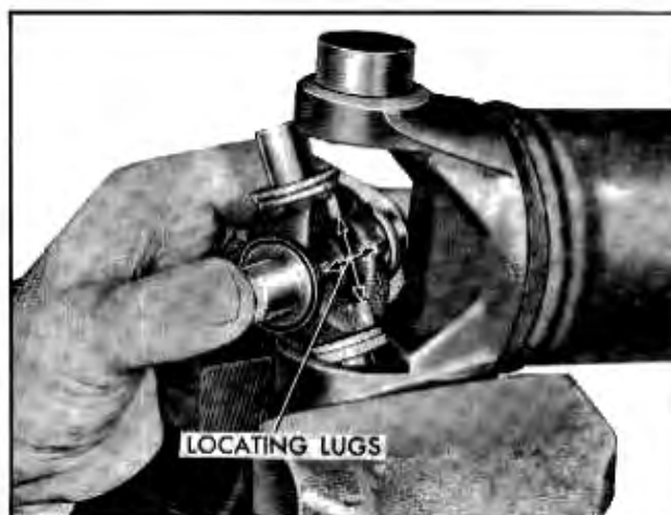
Fig. 4-50 Correct Installation of Journal in Yoke
