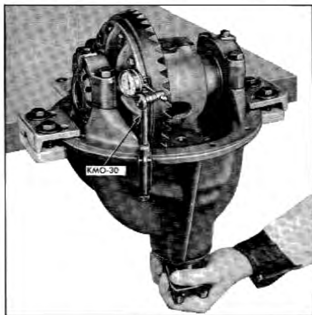
Fig. 4-12 Checking Ring Gear Run-out With KMO-30 Set
