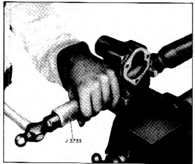
Fig. 9-16 Replacing Bearing Cup in Steering Gear Housing
