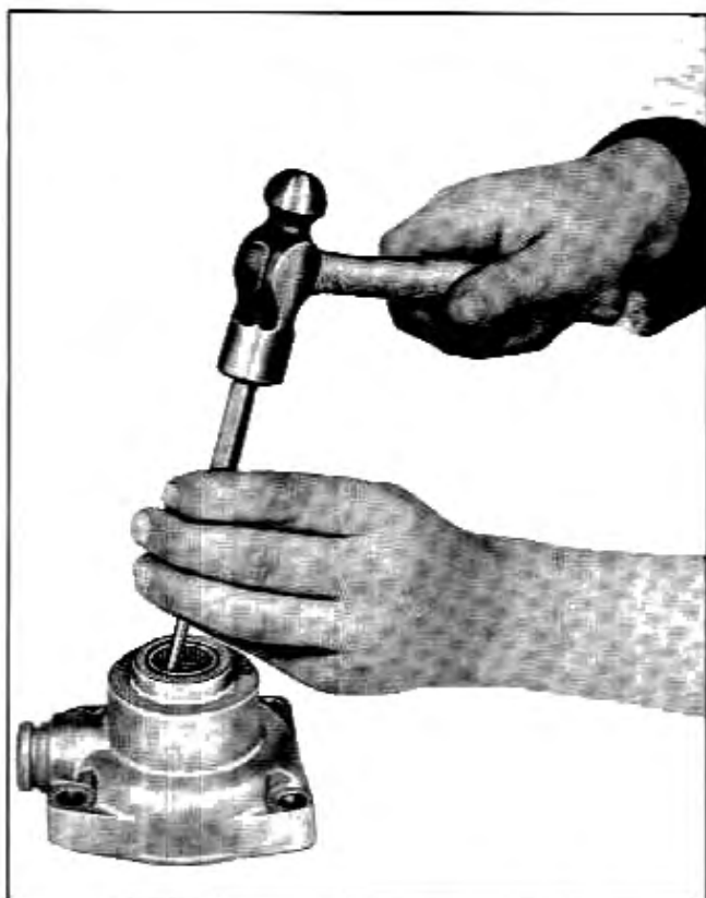
Fig. 9-43 Removing Housing Top Cover Oil Seal
