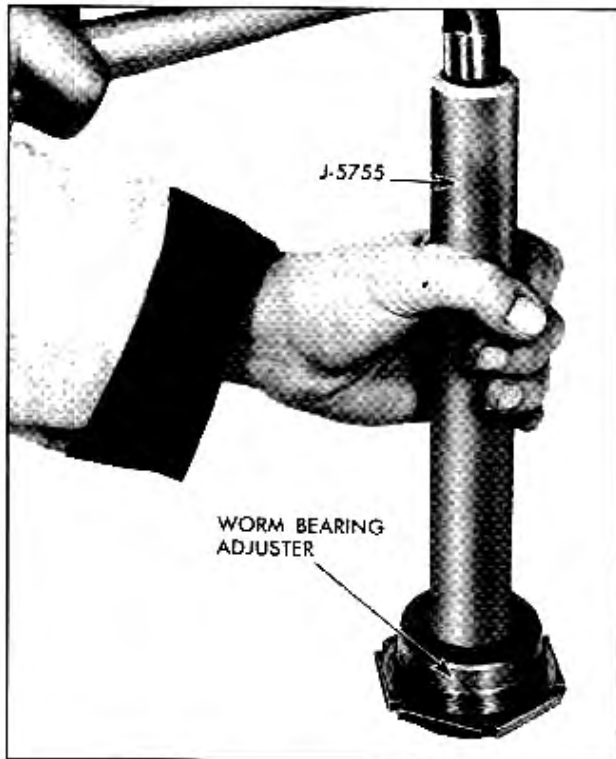
Fig. 9-15 Replacing Bearing Cup in Worm Bearing Adjuster
