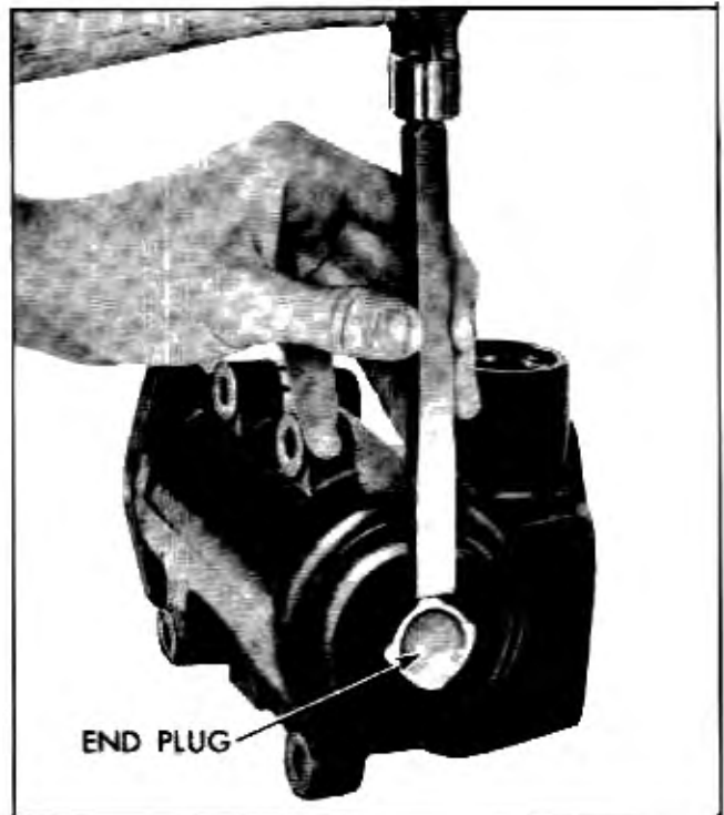
Fig. 9-47 Removing Housing End Plug Staked Portions
