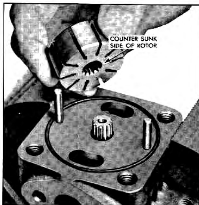
Fig. 9-76 Removing Pump Rotor
