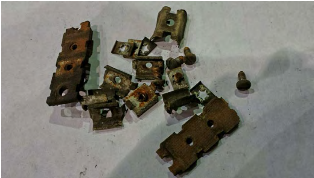
Crumbly original terminal block during disassembly.
