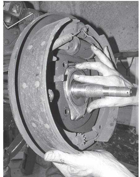
Before we replaced the brake drum, we elected to repack both the inner and outer wheel bearings. The outer bearing set came out before the drum was removed. The inner bearings need to be tapped out from the inside of the drum. The wheel bearing seal will drop out at the same time.
