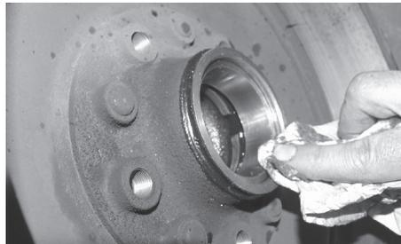
Thoroughly clean the bearings in solvent and then blow dry with compressed air. Never spin the bearings with compressed air, doing so runs the risk of nicking the rollers. To pack them, put a wad of appropriate high-temp axle grease in the palm of your CLEAN hand and push the bearing through it several times, as shown. Work the grease through the bearing rollers, and continue until it oozes out the other side.
