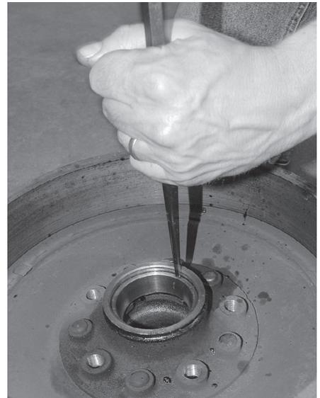
After cleaning and checking the bearing race (the bearing contact surface pressed into the hub) for wear or burn marks (blueing of the metal) and finding them okay, we lightly tapped it, alternating from side to side, back toward the outside of the hub.
