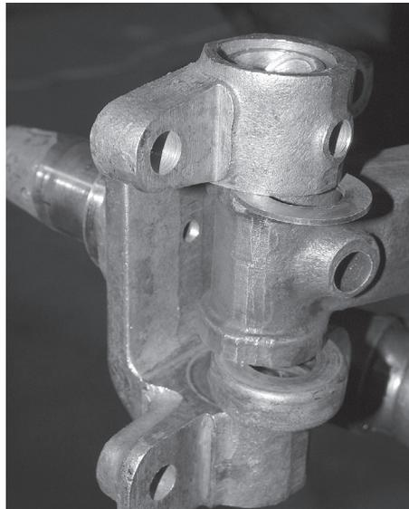
With the bushings in place, we were ready to re-assemble. Here, all the new parts are ready to install, including new bushings pressed in place, king pins (notched where the new lock pin will hold it into place), spacers, thrust bearings, grease fittings and end caps.
