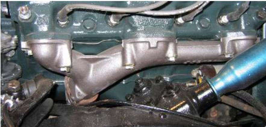
57 and 58 driver's side manifolds are the same. Note how the manifold exits to the front to clear the steering box. This is the adaptor Rick mentioned that directs exhaust to the rear.
