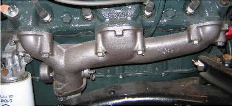
1957 through 1960 passenger side exhaust manifolds are interchangeable.
