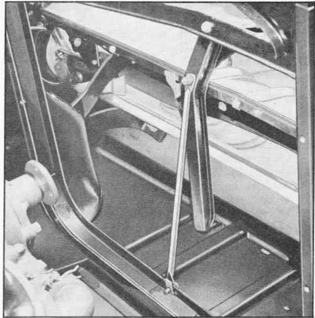
Fig. 4 Reinforcement Assembly #521158 Installed (Radiator Removed to Facilitate Photography)
