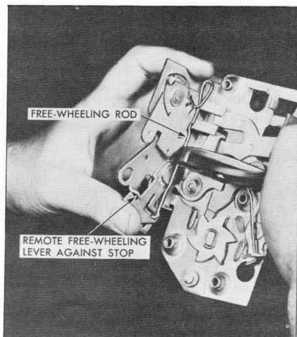
Fig. 7 Kinking Free-Wheeling Rod
