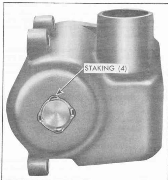
Fig. 49 Housing End Plug Staked
