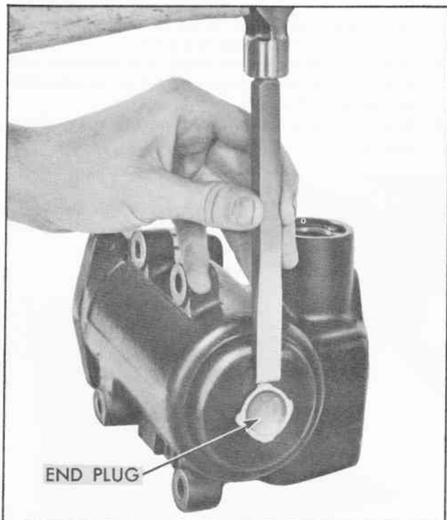
Fig. 48 Removing Housing End Plug Staked Portions
