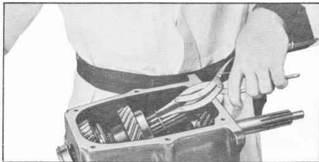
Fig. 24 Removing Second Speed Gear Snap Ring
