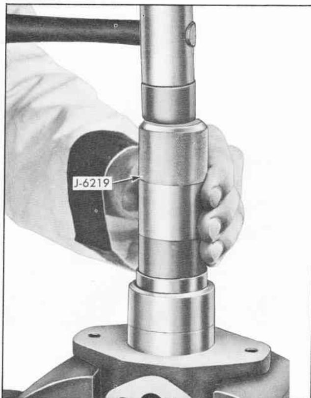
Fig. 108 Driving Shaft and Bearing Into Pump Body
