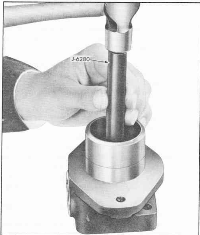
Fig. 106 Driving Needle Bearing Into Pump Body
