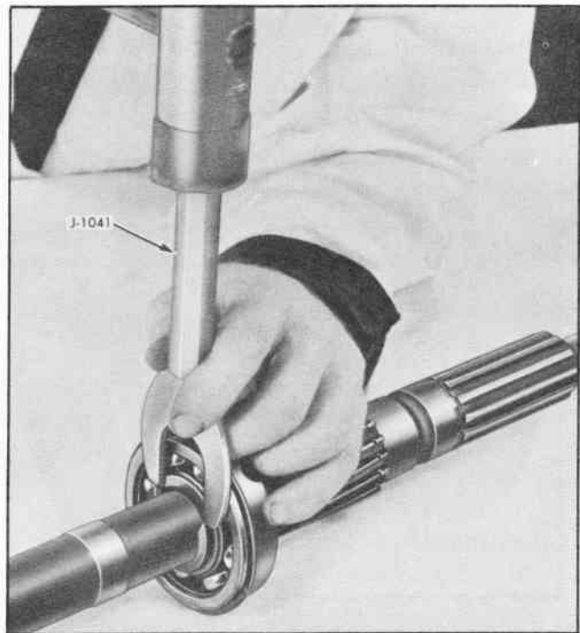
Fig. 34 Removing Rear Bearing Snap Ring
