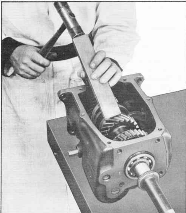
Fig. 22 Freeing Transmission Rear Bearing from Case
