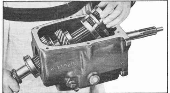
Fig. 23 Removing Synchronizer from Main Shaft
